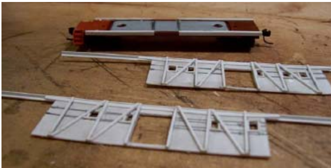
Additional styrene "L" angle was added to the under frame to support the caboose sides. The center sections on both sides were left out to have room for the baggage doors that would be added later.
