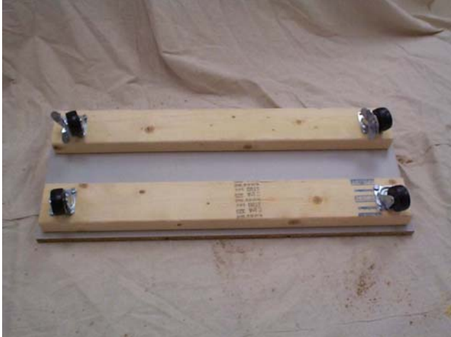
Here is a photo of the underside of the bottom panel with the 2 x 4s and casters.
