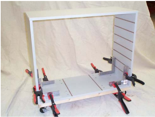
This photo shows the box of the organizer after it was glued and clamped together.
